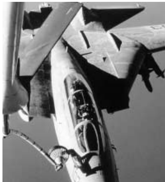
The modern Air Force uses both the flying-boom (above) and probe-and-drogue (below) methods of air refueling. The flying boom transfers fuel rapidly but can service only one aircraft at a time. In contrast, the probe and drogue, used by Navy aircraft, fuels too slowly for large bombers but can accommodate multiple aircraft simultaneously.
