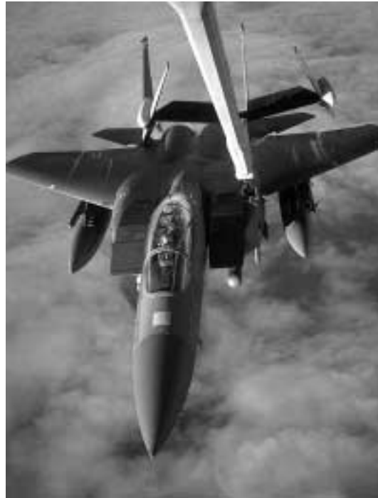
The modern Air Force uses both the flying-boom (above) and probe-and-drogue (below) methods of air refueling. The flying boom transfers fuel rapidly but can service only one aircraft at a time. In contrast, the probe and drogue, used by Navy aircraft, fuels too slowly for large bombers but can accommodate multiple aircraft simultaneously.
