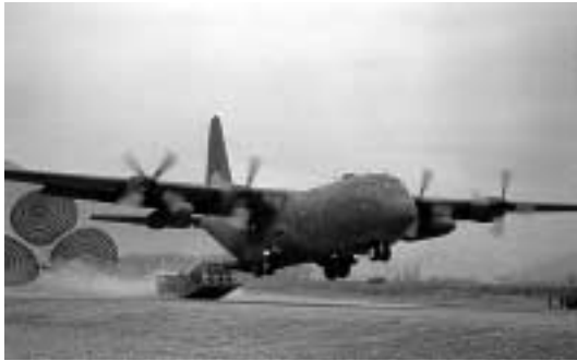
The venerable C-130, here making a low altitude parachute extraction system (LAPES) delivery to a forward location, has been in production continuously since 1956. Much smaller but more numerous than the C-17, the C-130 has its engines on the high wing, making it less vulnerable to FOD when it operates on unpaved runways.
